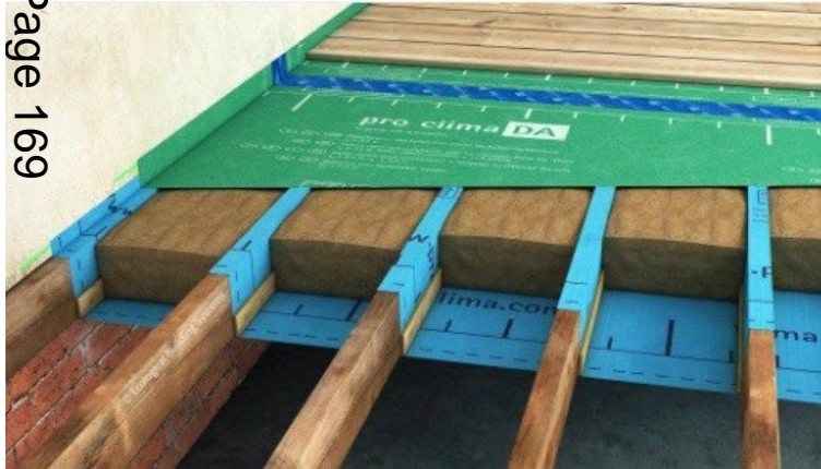
Insulated ventilated timber floor using hydroscopic insulation and breathable membrane (Ecological Solutions)
